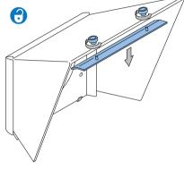
2. Carefully position the glass panel on the bottom glazing bar inside the hood
