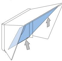
3. With the glass supported at all times, replace the top glazing bar and secure with the two screw fixings.
