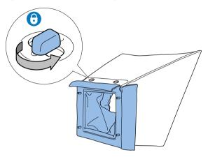
**4.** Align the single eyelets in both the side flags with the tabs and twist to lock.
