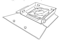
When used for outside broadcasts and other portable applications, the hoods can easily be folded flat again for transportation.
