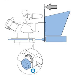
2. Tighten the rod clamps to secure the assembly in position.
