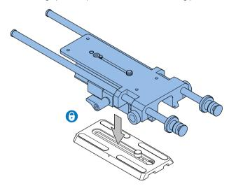
2. Fit the MT-BLUE mounting plate to the camera support.
