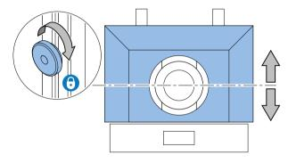
2. Adjust the vertical position of the hood to centralise it with the camera lens and fully re-tighten the fixing screws.
