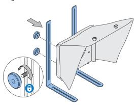
7. Fit the support bar onto the brackets and secure with the two locking knobs ensuring the bar is in a central position.
