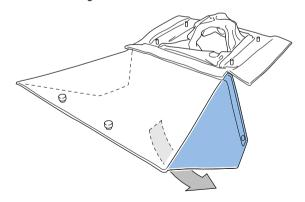
**3.** Align the two eyelets in the top flag with the tabs and twist to lock.
