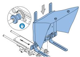
2. Loosen the rod clamps on the MT-BLUE mounting plate and slide the hood assembly fully forwards.
